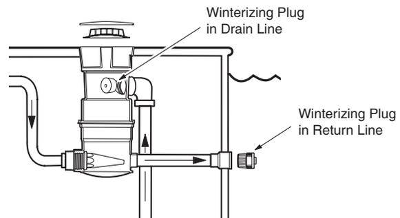
4. Close the valve at the pool equipment. Open the tee in the supply line and blow out the line.
